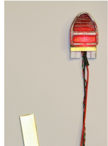
A slot in the mounting block takes the 6mm wide stalk.
